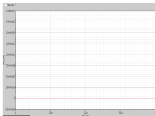
Fig. 8 Static power dissipation of Sub-Threshold 10T SRAM cell.
